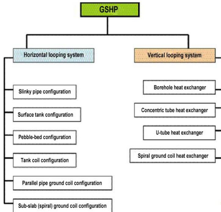
Figure 7: Common types of ground-loop heat exchangers [8]
