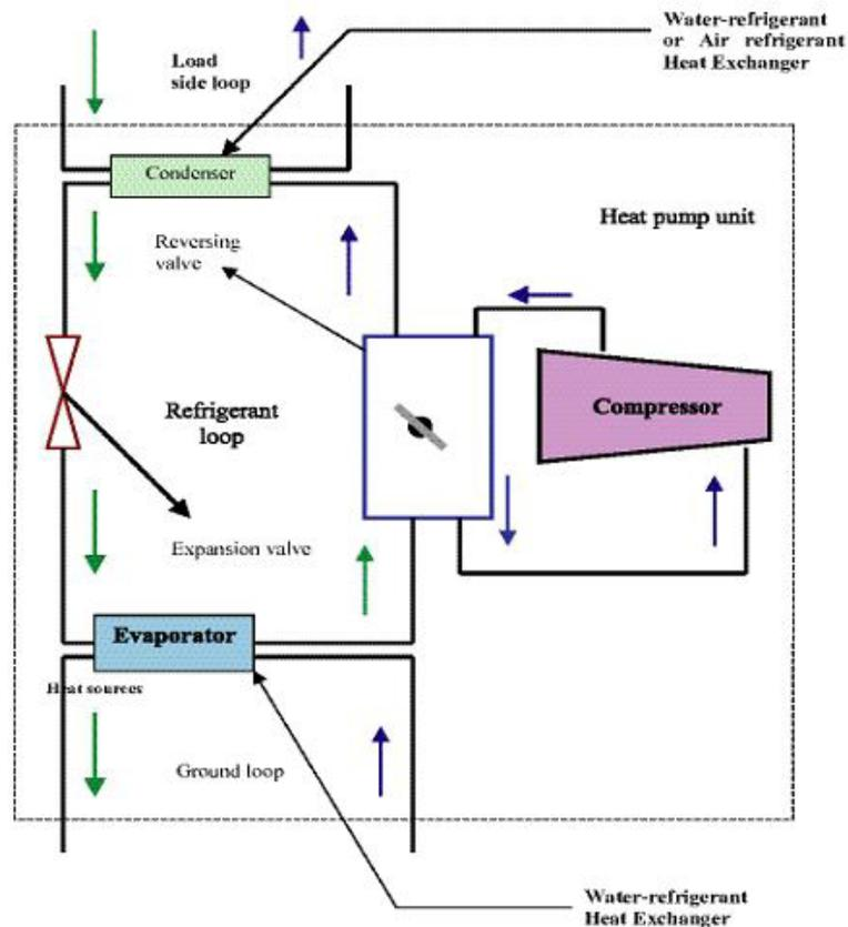
Figure 8: Schematic of GSHP system (heating mode operation)
